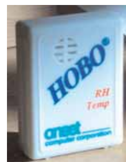
Hobo loggers monitor temperature and humidity
